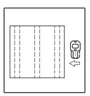
3 Using a stud finder, locate and mark the studs for strongest anchorage points.
